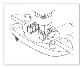
STEP 4 Secure the top using (1) #8 x 5/8" screw.\*
