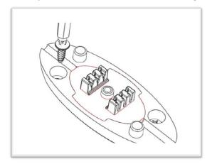
STEP 3 Being sure to line up wire colors use Punch-down tool to seat the remaining wires.
