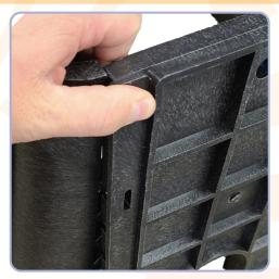
While still securing the top dovetail joint with your fingers, firmly knock the bottom of the short panel with the palm of your hand or using a rubber mallet. This will seat the rest of the joints locking it into place.
